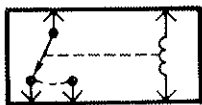
RELAY SHOWN WHEN COIL IS WITH NO CURRENT ENERGIZED, SWITCH FLOWING THROUGH IS PULLED CLOSED COIL
